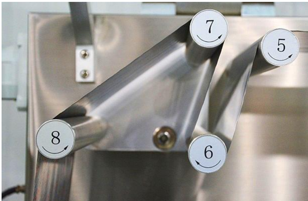
10. All of the guide rollers are labeled with a sequence number and placement direction, making it very easy to guide the film and lid foil through the machine.
