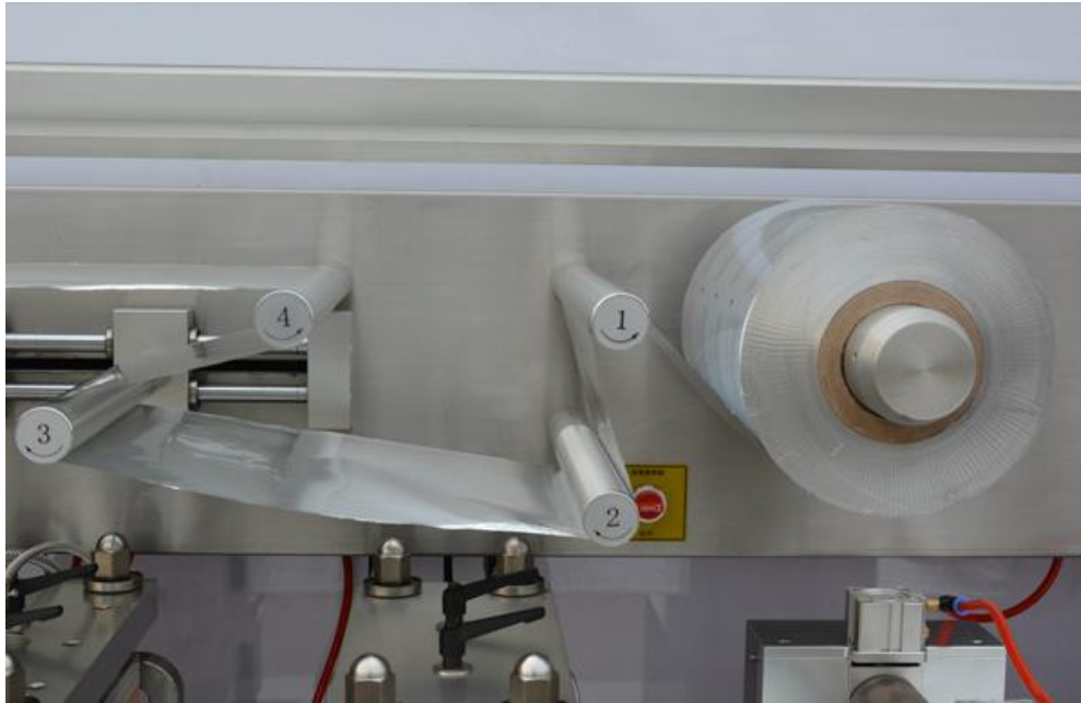
9. The lidding material loader adopts a fast lock mechanism, enabling replacement of lidding material easily within about 10 seconds.
